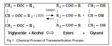
Transesterification is the reaction of fat/oil triglycerides to fatty acid alkyl esters and low molecular weight alcohols in the presence of catalyst [13]- [14] as shown in Figure 1. Short-chain alcohols such as methanol, ethanol, and butanol are the
