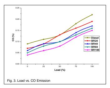
The graph shown in Figure 4 indicates that neat biodiesel has low CO emission and diesel has the highest in comparison to all the RBOME blends. CO is mainly formed due to the lack of oxygen and biodiesel is an oxygenated fuel, so it leads to enhanced fuel combustion that resulting in the decrease in CO emission.
